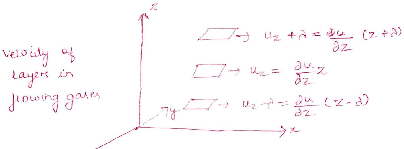
Imagining two imaginary large parallel flat plates, one lying in the  $xy$ -plane, the other at a distance  $z$  above the  $xy$ -plane.
